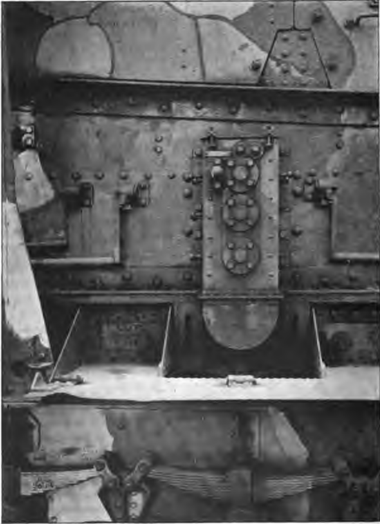
CAR TRAVERSING MECHANISM OF THE 280-MM. GERMAN GUN MOUNT (GEAR CASE ON LEFT SIDE OF MOUNT).
